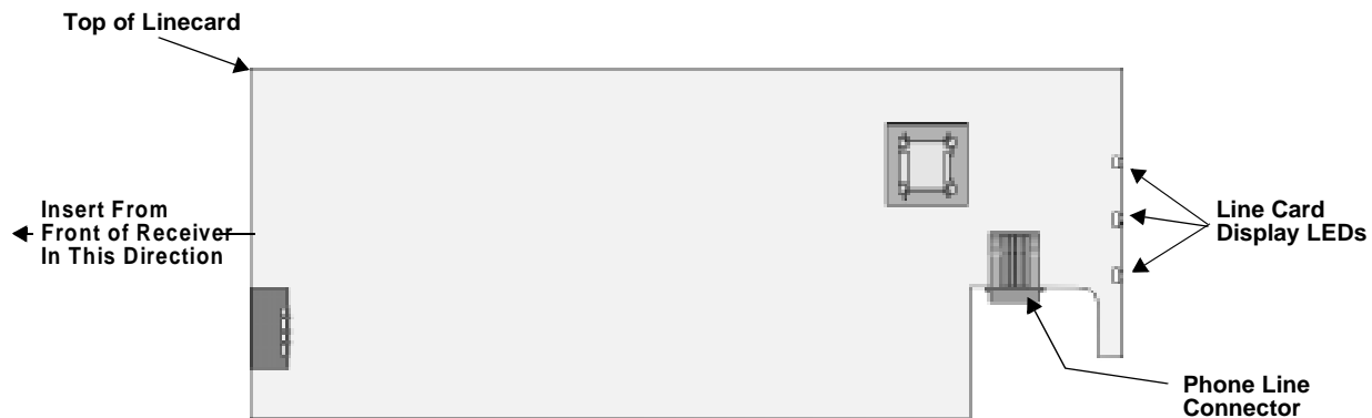
Figure 3-6 Line Card Position and Components
